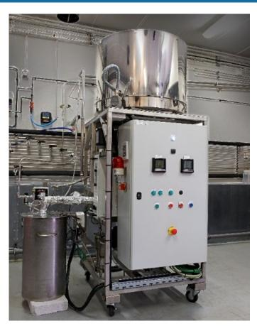
(co-)electrolyzer module developed by CEA
