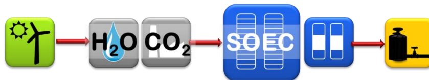
Figure 1. ECo approach of using electricity from fluctuating sources like wind and solar, together with steam, and CO 2 from sources like biogas or the cement industry in the SOEC process, yielding synthesis gas, which is converted in a catalytic unit to hydrocarbons like methane, which in turn can be added to the existing natural gas infra structure
